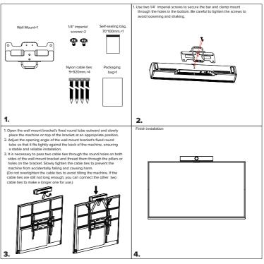
Safety warning: When using the Clamp mount, be sure to use nylon cable ties. Thread them through the safety holes of the clamp mount and tie them to the mounting hole of the bracket (or the VESA rivet of the IFP). This will keep the NEXT from falling off the top of the IFP.
